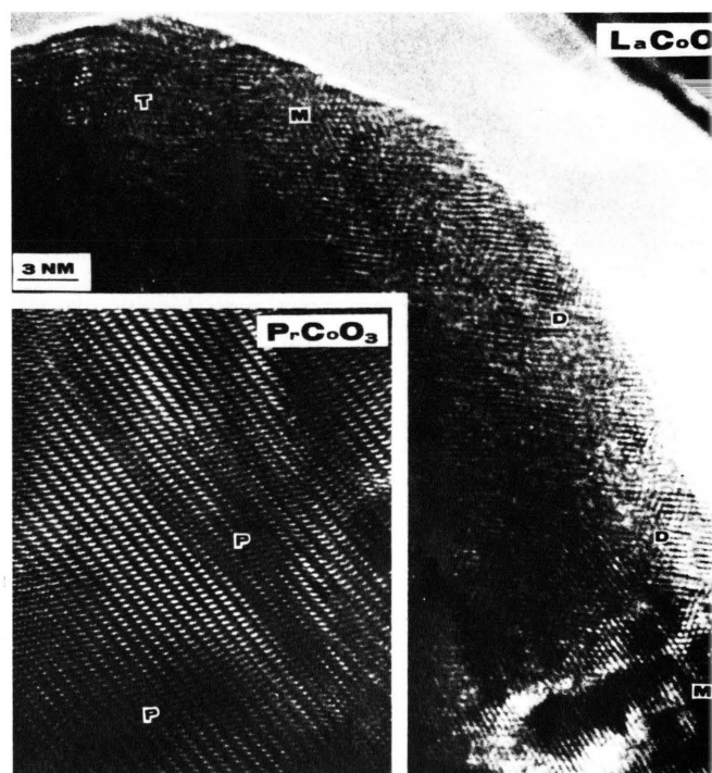
Fig. 10. The planar faults in \text{PrCoO}_3 catalyst.
